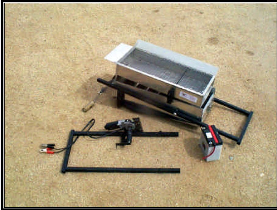
Insert back legs onto the riffle tray.
