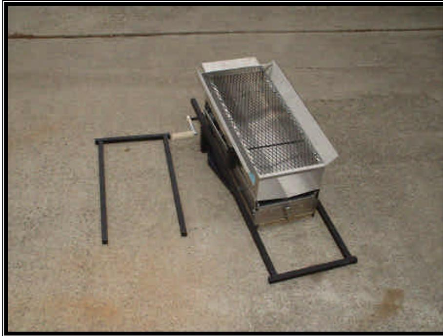
Insert back legs into sockets in back leg holder. Be careful not to get the bellows cloth caught between the legs and the leg holder.
