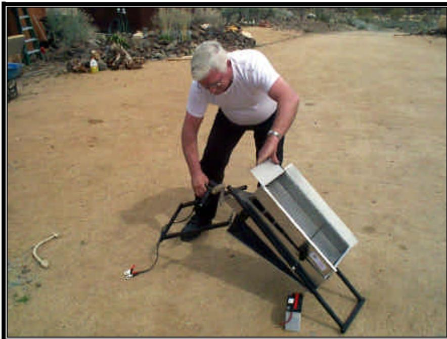
Lift the top box up and insert the front legs.
