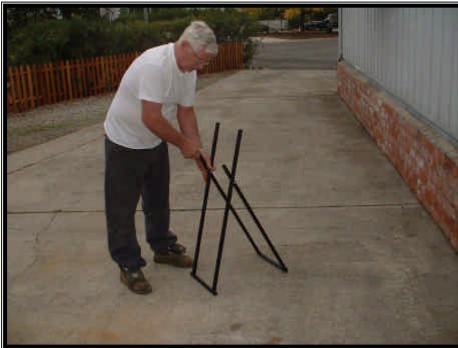
Set the drywasher on the legs with the front part of the top box on the long legs (as shown).
